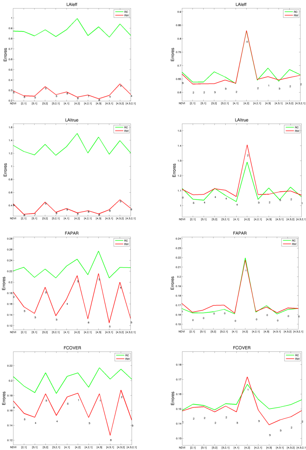
Figure 13: Test of multiple regression (Transfer Function) applied on different band combinations. Band combinations are given in abscissa (2=G, 3=RED, 4=NIR and 5=SWIR). The weighted root mean square error (RMSE) is presented in red along with the cross-validation RMSE in green. The numbers indicate the number of data used for the robust regression with a weight lower than 0.7 that could be considered as outliers. Left: First campaign (May). Right: Second campaign (June).
