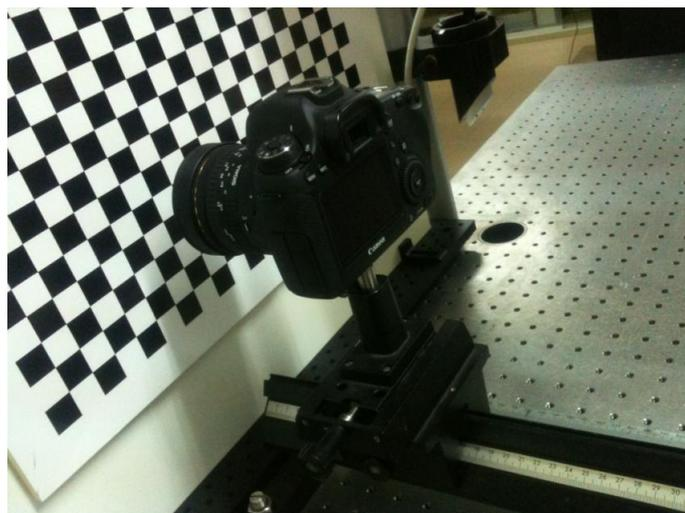
Figure 6: Alignment of the system formed by the camera + sigma lens.
